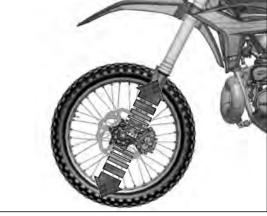
Tighten the wheel bolt and the screws of the foot-leg.
