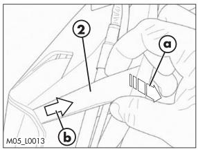
Remove the jumper 2 by pulling the rear portion towards you and slide it towards the rear.
