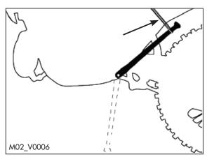
If the vehicle is used off-road, the closed stand can be further fastened by means of rubber band.
