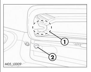
To re-assemble: Insert the cavity  ${\bf 1}$  of the saddle in slot  ${\bf 2}$ .
