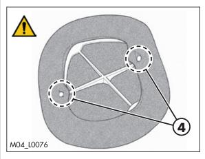
• To hook the inside edges of the filter with the correspondents grafts **4** found on the cage.
