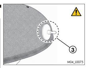
• To completely insert the rungs **3** of the cage into the filter seats.
