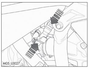
Connect the fuel connections by coupling them completely.
