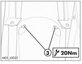
Remove the screws 3, 4 and 5 (one for each side) fixing the mudguard to the vehicle.
