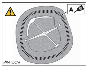
Note: before refitting the filter to the vehicle is recommended to apply a long-term grease in the area **A**.
