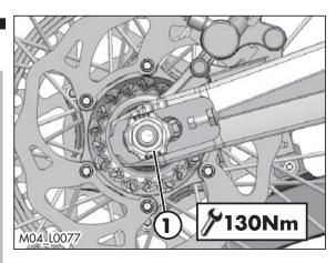
• Tighten the pin 1 to the torque indicated.
