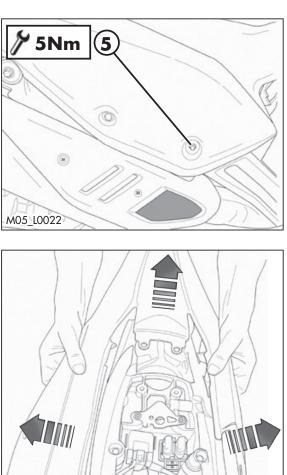
Grasp the mudguard by the sides, spread the fender and slide out towards the rear.
