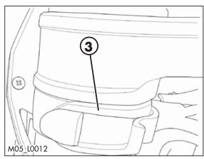
Pull the mask upwards and rotate it forward from the top.
