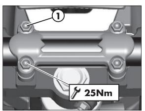
To adjust the position of the u-bolt remove the screws shown in the figure.
