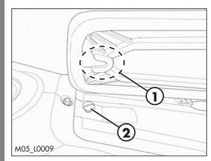
To re-assemble: Insert the cavity **1** of the saddle in slot **2**.
