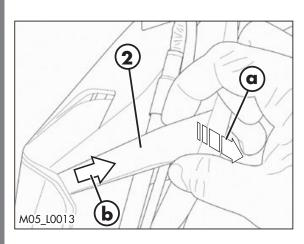
Remove the jumper 2 by pulling the rear portion towards you and slide it towards the rear.
