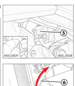
Lift the tank slightly and: • remove the tube **6**.
