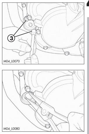
Mount the new paper filter, close the oil tap to engine, tighten the screws at 10 Nm.
