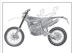
Press the saddle down in the middle and at the same time, push it forwards until the bayonet joint engages in its seat.
