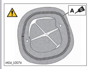
Note: before refitting the filter to the vehicle is recommended to apply a long-term grease in the area  $\mathbf{A}$ .
