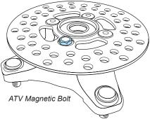
The magnet spins around tripping the sensor switch each time--giving Voyager speed, distance and time data to compare with the GPS data.
