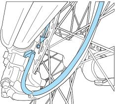
Magnet Passing Under Sensor Voyager can tell precisely how far and fast it's traveled by how many times the magnet passes the sensor.
