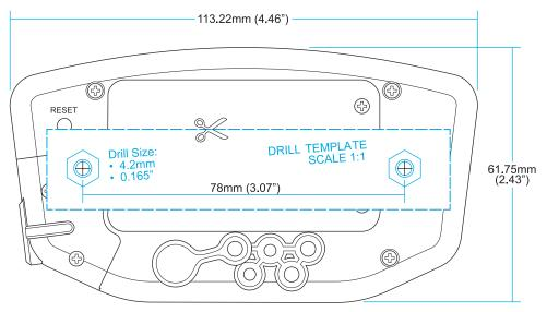
Use the included M4x16 bolts to mount to any flat surface. If other than provided screws are used, make sure they are not too long for mounting holes or they will damage internal components of Voyager.
