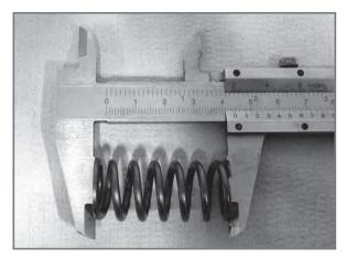
Clutch spring length measurement.
