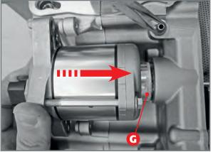
Insertion of start motor in crankcase half. Note zone G to be greased.
