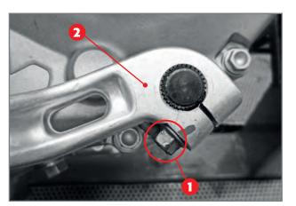
Removal of gear lever.
