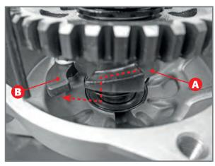
Positioning of sleeve A below ramp B.
