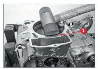
Disassembly of crankcase.
