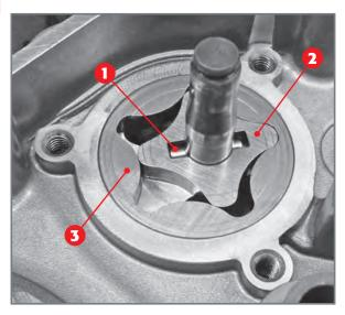
Coupling high-pressure pump rotors to drive shaft.
