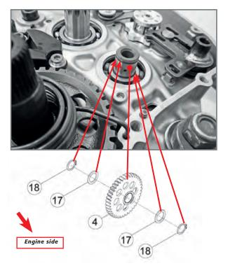
Kickstart device unit coupled to the crankcase.
