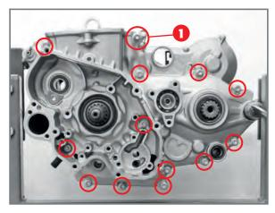
Screws 1 for blocking left side casing.
