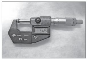
Use of the digital micrometer to measure the calibrated discs.
