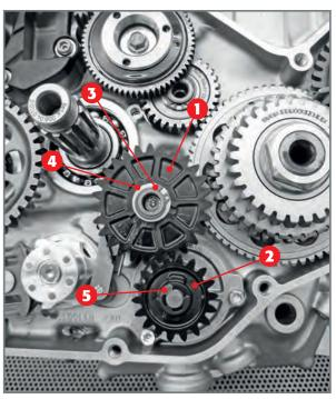
Gear unit for oil pump control.
