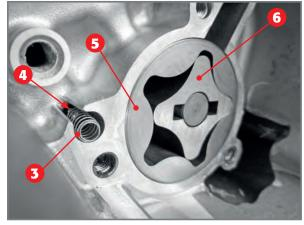
Low-pressure oil pump and by-pass valve.
