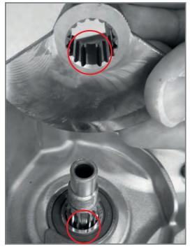
Detail of grooved profiles for coupling.
