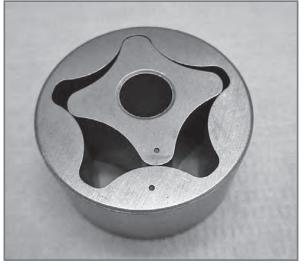
Low pressure pump: note the dot on the two rotors. The dot must face the inside of the engine.
