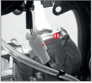
Disconnect the rear brake stop connector 11.
