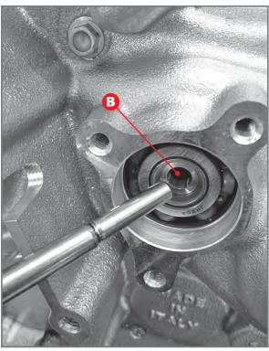
Insertion of clutch rod in housing B.
