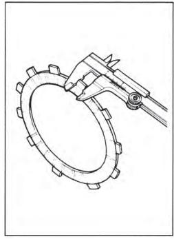
Minimum disc tooth thickness.
