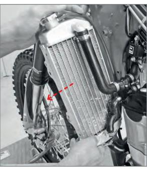
Remove the left radiator with pipes.
