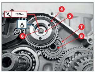
Coupling electrical starter gear unit.
