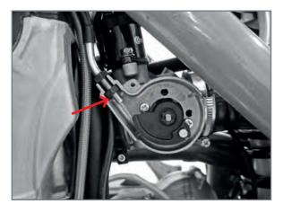
Set the gas cable on the left side of the frame and make it pass outside the head connection.
