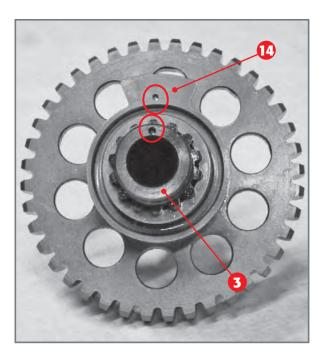
Positioning of sleeve on small shaft.
