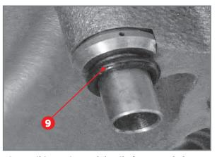
Piston oil jet O-ring and detail of passage hole.
