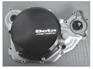
Complete internal clutch cove of water pump.
