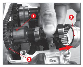
Removal of intake camshaft 1, bearing 2.
