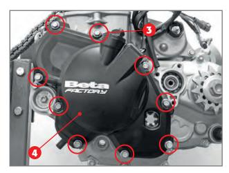
Fixing screws C of ignition cover D.
