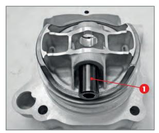
Application of pin bolt to piston.
