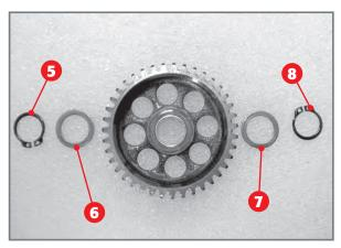
Two circlips 5 and 8 and thrust washers 6 and 7.
