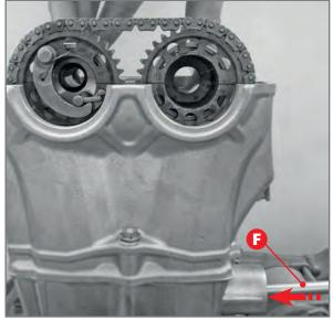
Phasing check. Note the pressure that the cylinder B exercises on the chain.
