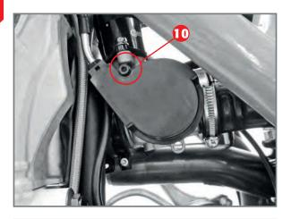
Remove the screw of the throttle body **10** cover and the cover itself.
