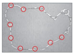
Positioning of M6x25 screws.
