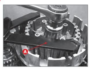
Removal of inner hub nut with relevant tool G.
