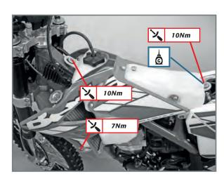
Grease the rear fastener and tighten the screws at the indicated torque values.
