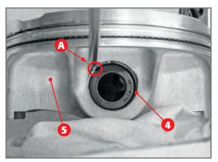
Removal of elastic ring 4 from right hand side of pi-
