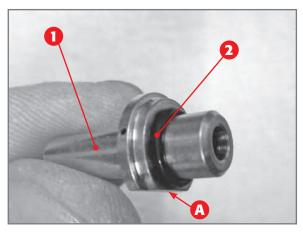
Oil jet with O-ring. Note the flat part A for reference on the side of the jet.
