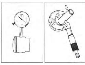
Measuring pin bolt seat and pin bolt.
