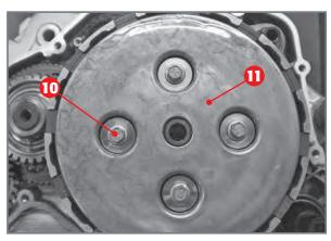
Clutch cap 11 and four screws 10.
