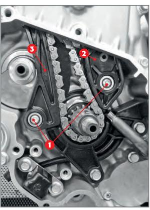
Fixing screws 1 of mobile 2 and fixed pad 3.
