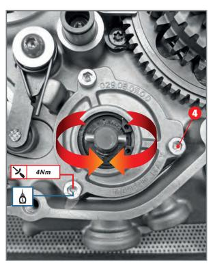
Coupling high-pressure pump cover to crankcase.
