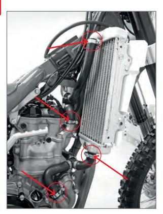
Disconnect the water hoses from the engine and from the right radiator.
