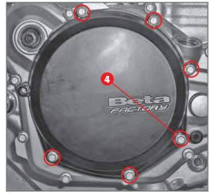
4 screws that fasten the outer clutch cover to the inner cover.
