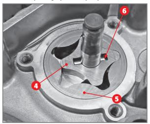
High-pressure pump. 4) Internal rotor; 5) External rotor; 6) Roller.
