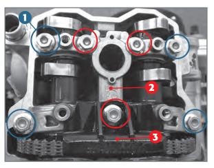
Fixing screws 1 camshaft support 2 and chain guide 3 The four outer screws circled blue must be taken off-
