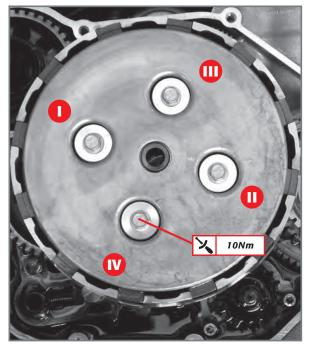
Complete clutch and recommended tightening order.
