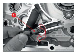
Disassembly of inner filter.
