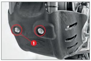
Back engine guard fixing screws.
