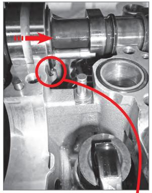
Positioning camshaft bearing.
