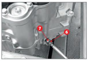
The crankshaft blocking screw 6 with copper washer
