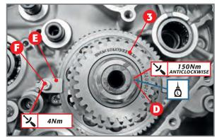
Coupling main gear to crankshaft.
