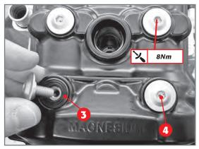
Application of rubber rings 3 and fixing screws 4.
