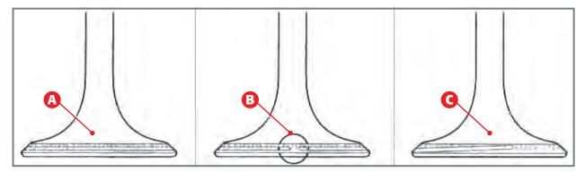
Valve-seat contact conditions: A) Correct; B) Incorrect - contact face damaged-; C) Incorrect - uneven width-.
