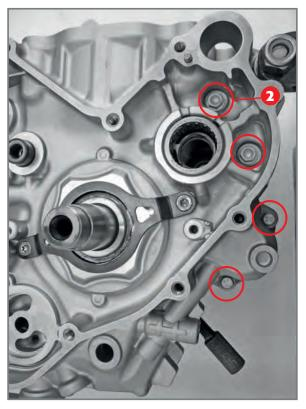
Screws 2 for blocking right side casing.
