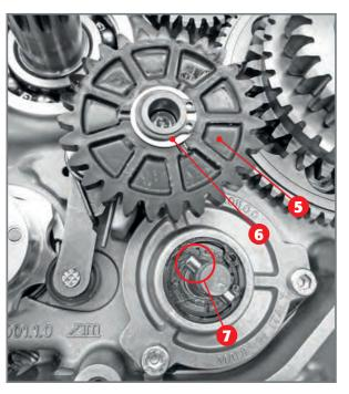
Coupling pump control gearwheels to crankcase.
