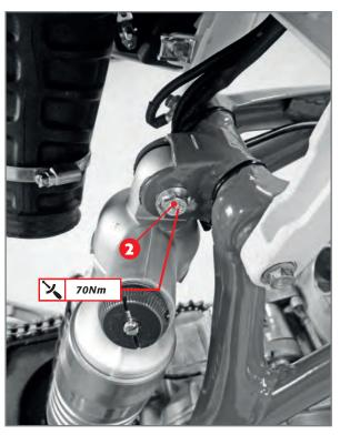
Insertion of upper shock absorber pin.
