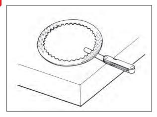
Measuring steel disc distortion.
