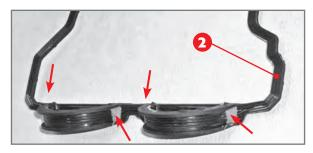
Edges where the gasket paste must be applied.
