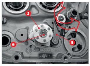
Disassembly of stop cam.
