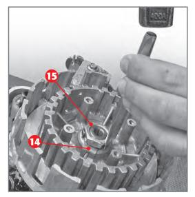
Opening safety washer with chisel.
