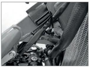
Electric connectors in the recess (injection versions).
