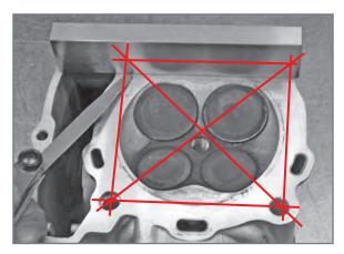
Checking flatness of cylinder head.
