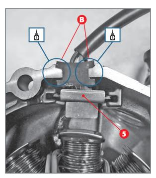
Application of cable protection plate 5. Note the two zones B where a drop of gasket paste must be applied.
