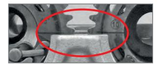
Detail of correct alignment of engraved notches on gearwheels of camshafts.
