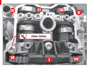
Tightening order of camshaft support screws.
