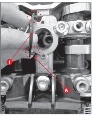
Application of spark plug gasket.
