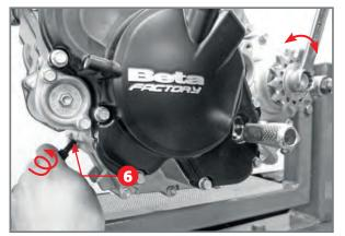
Securing of the motor shaft on the TDC. Make a note of locking screw 6 and the torque applied on the output shaft using a wrench.
