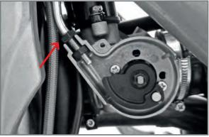
Loosen the adjustment nuts and release the gas cables.
