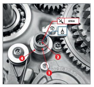
Oil pumps control gearwheels support pins.
