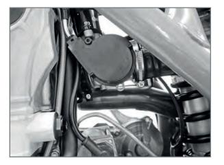
Apply the throttle body cover and the relative screw. Connect the stop connectors.
