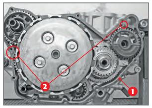
Positioning of gasket 1 and centring pins 2.
