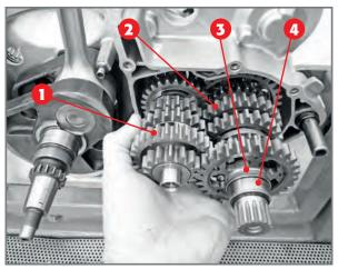
Insertion of gearbox in left crankcase.
