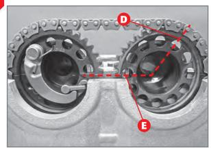
Positioning intake camshaft.
