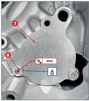
Coupling low pressure pump cover to crankcase.
