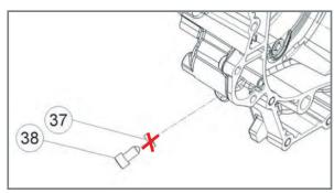
To block the crankshaft, apply only the screw 38 to the crankcase.
