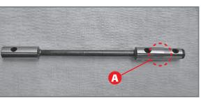
Also check that the drive shaft is not too marked in the zone A where the oil seal slides.
