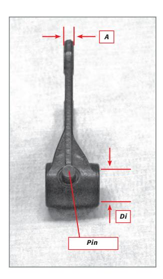
Make sure the distance **A** between the outer faces of the fork is not less than that indicated below:
