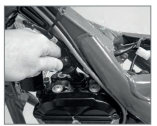
Disconnect the spark plug cap. Cut all straps binding the engine's electric system to the clutch pipe and to the frame.
