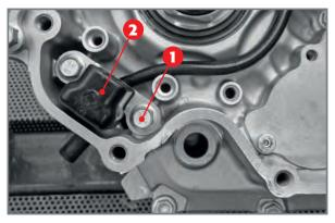
Two screws 2 for fixing pick-up 1.
