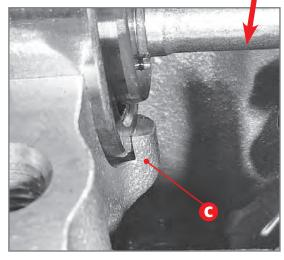
Detail of positioning bearing against shoulder C.
