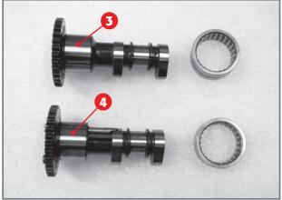
Camshafts (G intake, H exhaust) with bearings.
