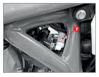
Disconnect the petrol pipe by pressing the relevant button of quick coupling 7.
