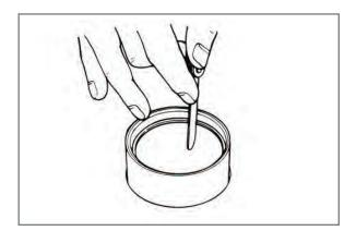
Checking the wear limit of the elastic band.
