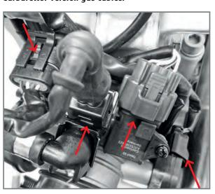
Disconnect the electric connectors indicated in the figure, relative to the throttle body.
