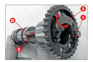
Check on the exhaust camshaft that the spring 1 of the centrifugal decompressor recalls the rest of the device so that the cylinder segment **D** of the rod 2 protrudes completely without any play.
