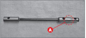
Checking oil pump control shaft.
