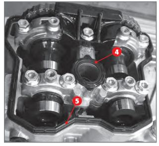
Spark plug gasket 4 and cylinder head cover gasket 5.
