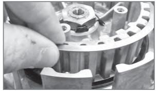
Removal of disc spring assembly.
