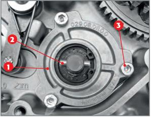
Disassembly of high-pressure pump cover.
