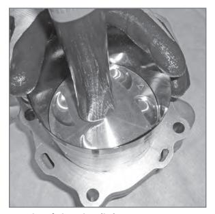
Insertion of piston in cylinder.
