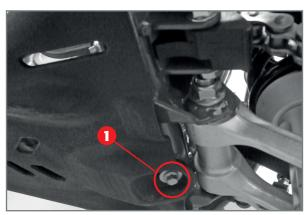
Front engine guard fixing screw.
