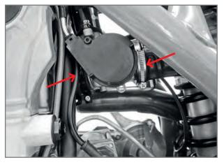
Loosen the throttle body straps from the air filter sleeve and from the manifold.
