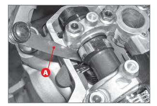
Checking valve play with thickness gauge.
