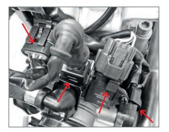
Connect the electric connectors indicated in the figure, relative to the throttle body.
