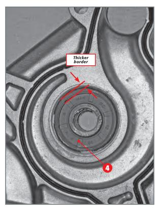
Application of oil seal on inner clutch cover.
