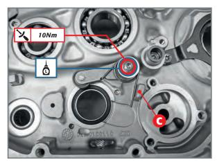
Stopping device coupled with the crankcase half.
