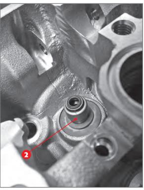
Insertion of valve stem seal.
