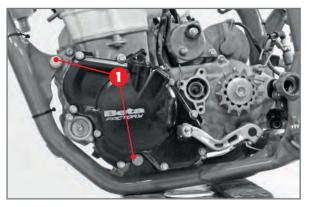
Insertion of engine pins.
