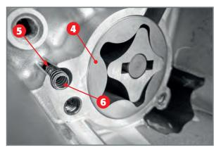
Complete low pressure pump coupled to the crankcase.
