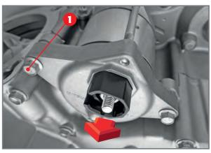
Screws 4 fixing start motor to crankcase.
