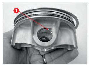
Application of circlip 1 to piston.
