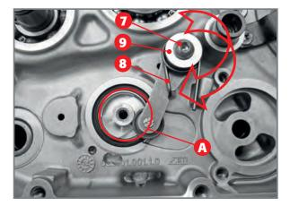
Disassembly of cam stop lever.
