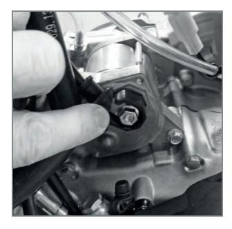
Remove the start motor cable fixing nut.
