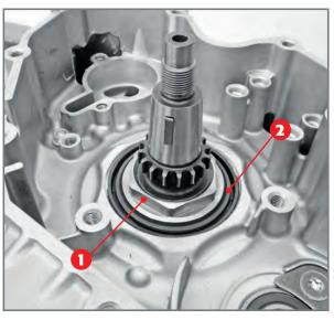
Nut B blocking crankshaft.
