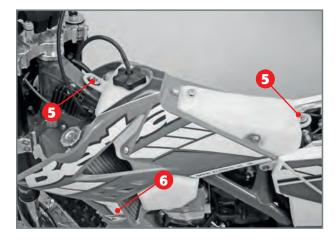
To dismount the tank, remove the seat, completely loosen the two screws 5 fixing the tank to the frame and screw 6 (one per side) which fixes the side to the radiator.
