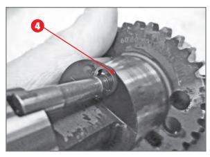
Extraction of Benzing ring from decompressor shaft.
