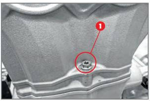
Chain-side head fixing screw.
