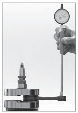
Bore meter verification of inside diameter of connecting rod foot.
