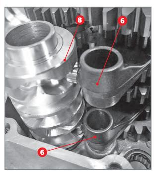
Positioning of the secondary unit forks 6 in the external guides of desmodromic device 8.
