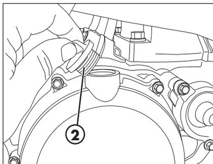
Use the oil indicated on page 16 in the "Recommended lubricants and liquids" table.
