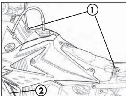
Remove the two screws **1** fastening the tank to the frame and the screw **2** (one per side) securing the fairing to the radiator.
