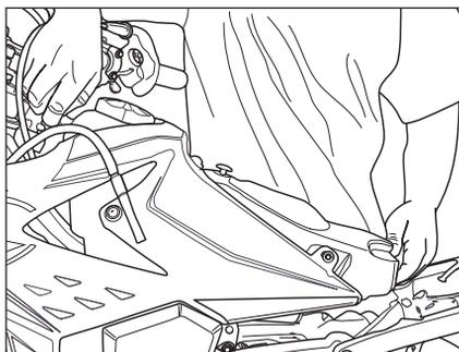
Lift the tank complete with side panels.
