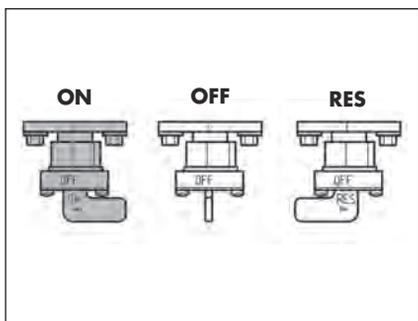
**OFF:** fuel supply closed. Fuel cannot pass from the tank to the carburettor.
