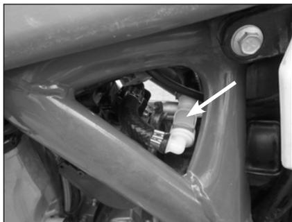
Disconnect the fuel hose by pressing the appropriate button of the quick coupling.
