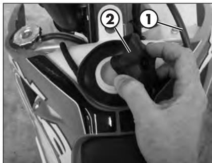
To close the fuel tank's cap, set it on the tank and crew it clockwise.
